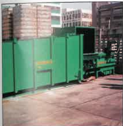
Superpak refuse compactor complete with bin lifter
